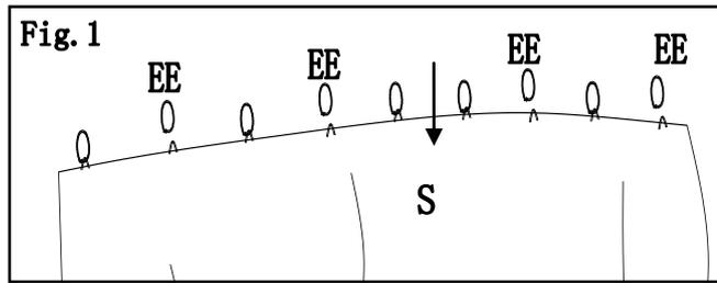
Fig.2: Fix the plastic ring (EE) to the short side curtain (S).
