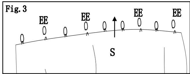
Fig.4: Take down the plastic ring (EE) from short side curtain (S).
