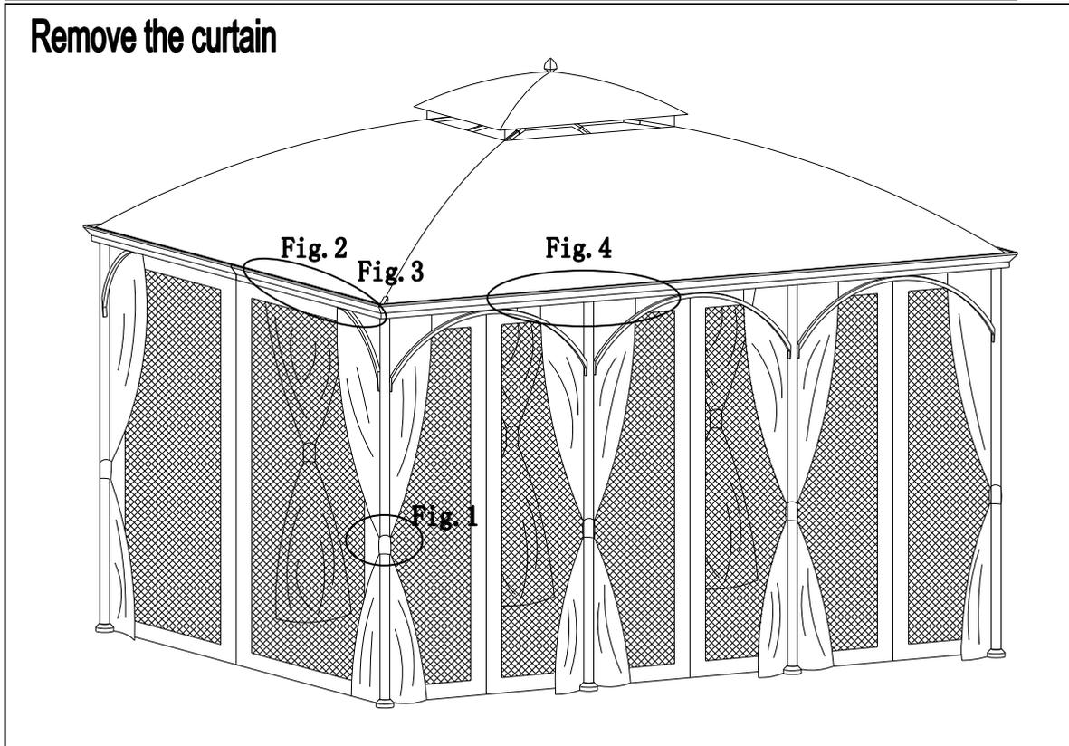
Fig.1: Open the hook-and-loop fastener at the curtain (S) which is tied on the post.
