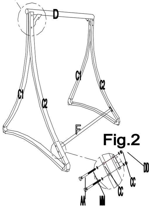
Step 3: Connect Top beam (D) to Front foot (C1) & Back foot (C2) by using bolt (FF), washer (GG) and nut (HH), then cover Plastic cap (EE), as Fig.1. Connect Foot connect bar (F) to Back foot (C2) by using bolt (MM), washer (CC), nut (DD), then cover Plastic cap (AA), as Fig.2.
