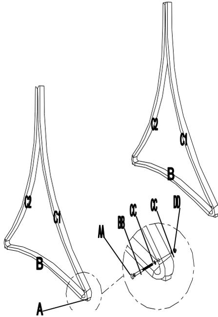
Step 2: Connect Foot connector (A) to Front foot (C1) & Back foot (C2) by using bolt (BB), washer (CC) and nut (DD), then cover Plastic cap (AA).
