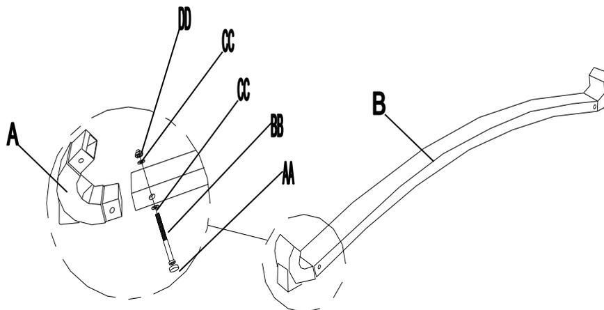
Step 1: Insert Foot connector (A) to Foot connect bar (B), fix them by bolt (BB), washer (CC) and nut (DD), then cover Plastic cap (AA).
