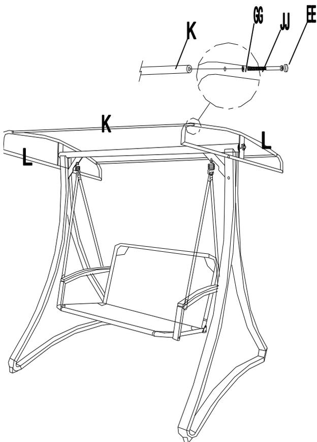
Step 9: Connect Top side support bar (L) and Top connect bar (K) by using bolt (JJ) and washer (GG), then cover plastic cap (EE).
