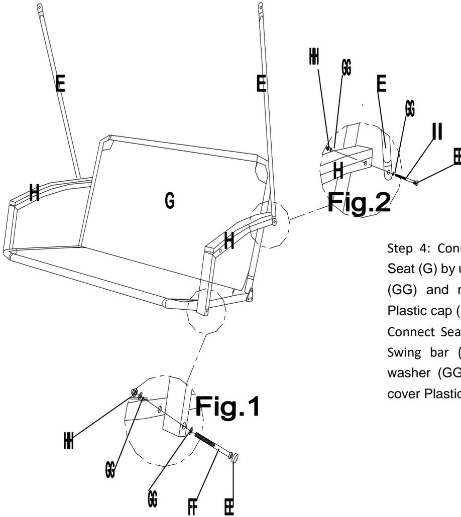
Step 4: Connect Armrest (H) and Seat (G) by using bolt (FF), washer (GG) and nut (HH), then cover Plastic cap (EE), as Fig.1.
