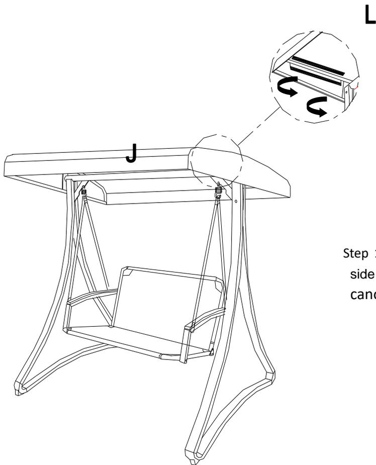
Step 10: Stretch the canopy to fit, wrap Top side support bar (L) as well and stick the canopy velcro.
