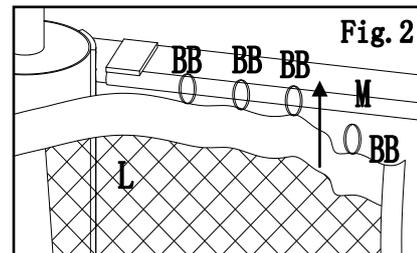
Fig.3: Draw the netting in by the buckle and elastic string and fix the netting to the post by tieback.
