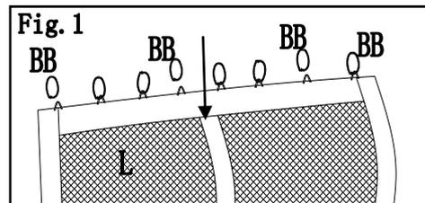
Fig.2: Hang the netting (L) to the netting pipe (M) by the plastic ring (BB).
