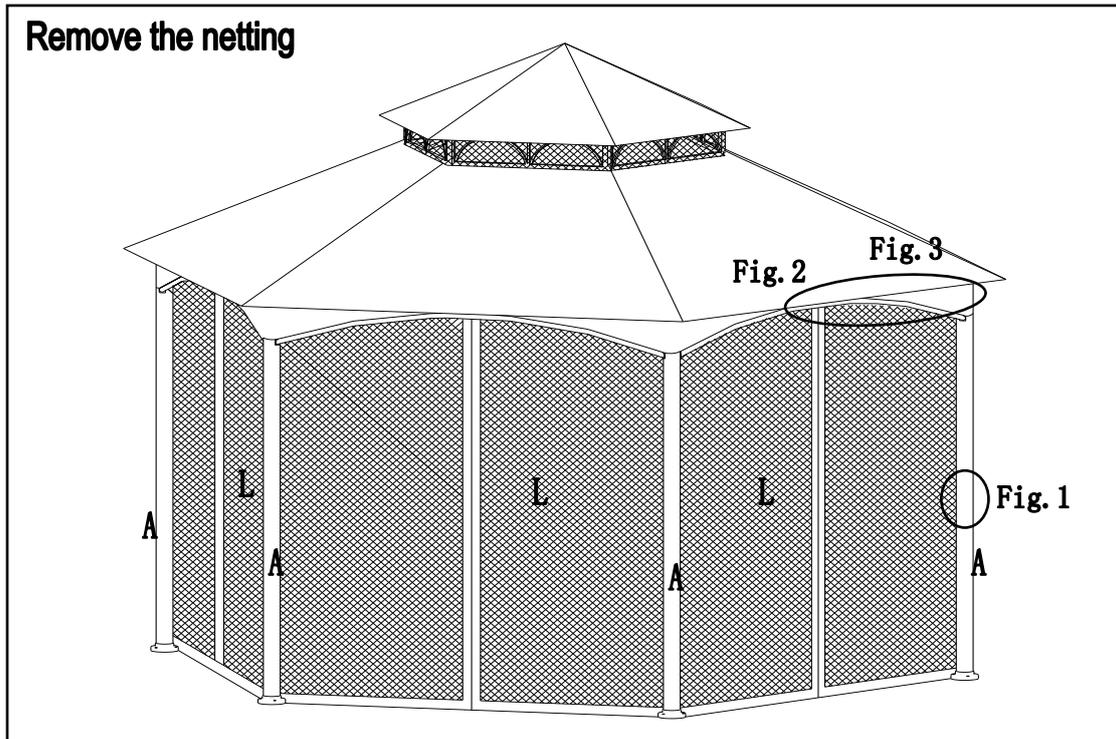
Fig.1: Loosen the tieback on the post and the buckle on the netting.
