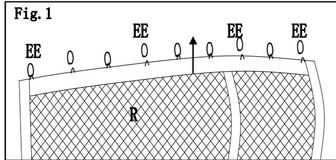
Fig.2: Fix the plastic ring (EE) to the short side of netting (R).
