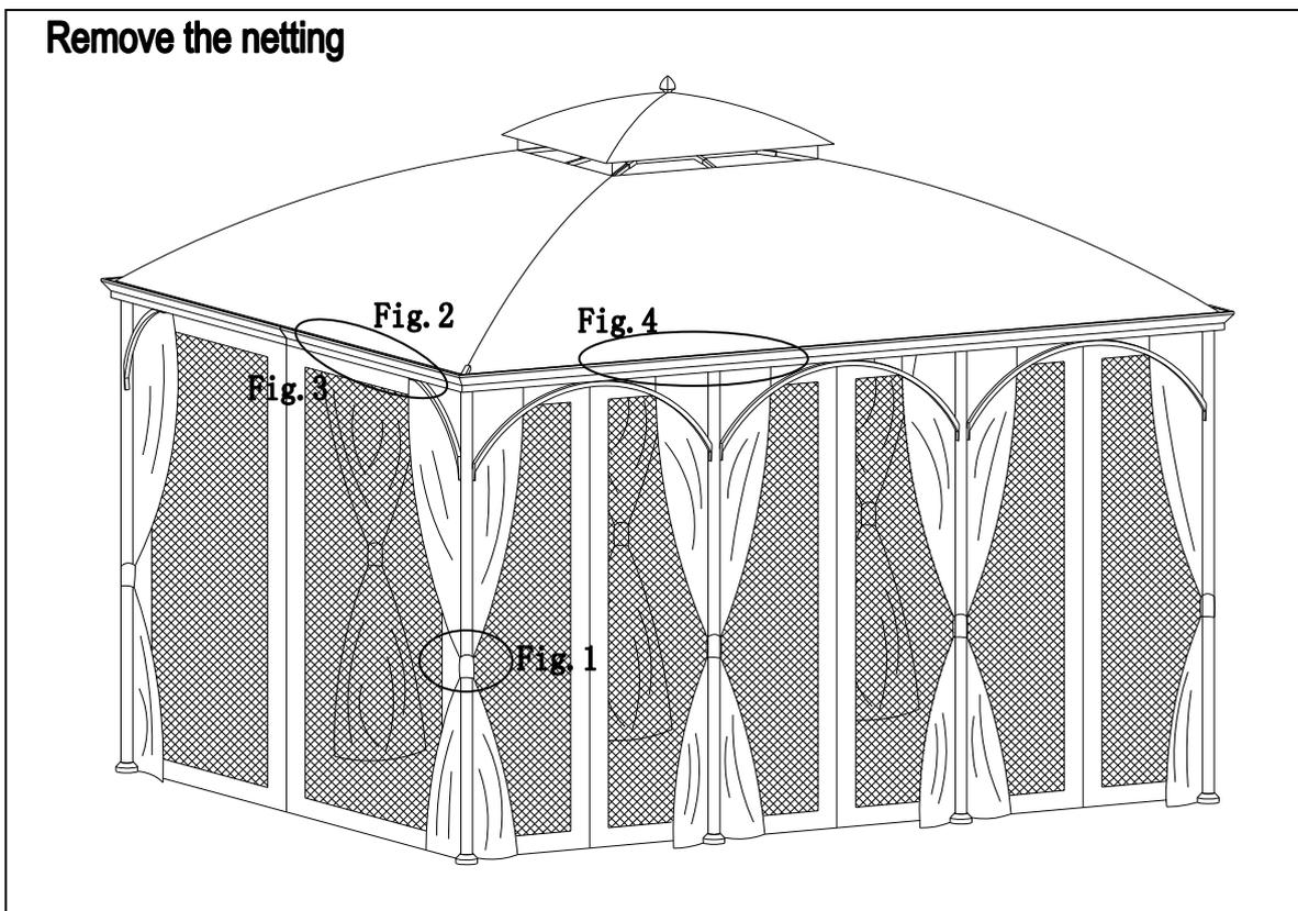
Fig.1: Open the hook-and-loop fasteners on the curtain (S) to release the netting (R).
