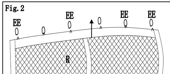
Fig.3: Hang the netting (R) to the netting pipe by plastic ring (EE). Please make sure short side contains 6 plastic rings and long side contains 3 plastic rings.
