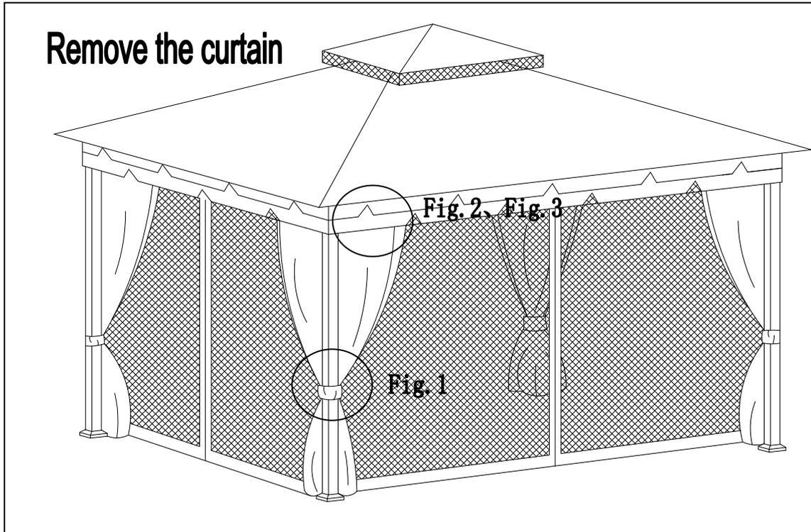
Fig.1: Loosen the tieback of the curtain (V) which is fixed on the post.
