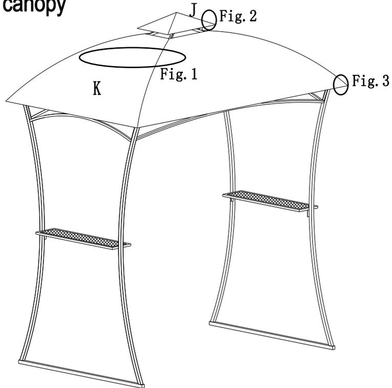
Fig.1: Put the big canopy (K) onto the big top but do not spread put.
