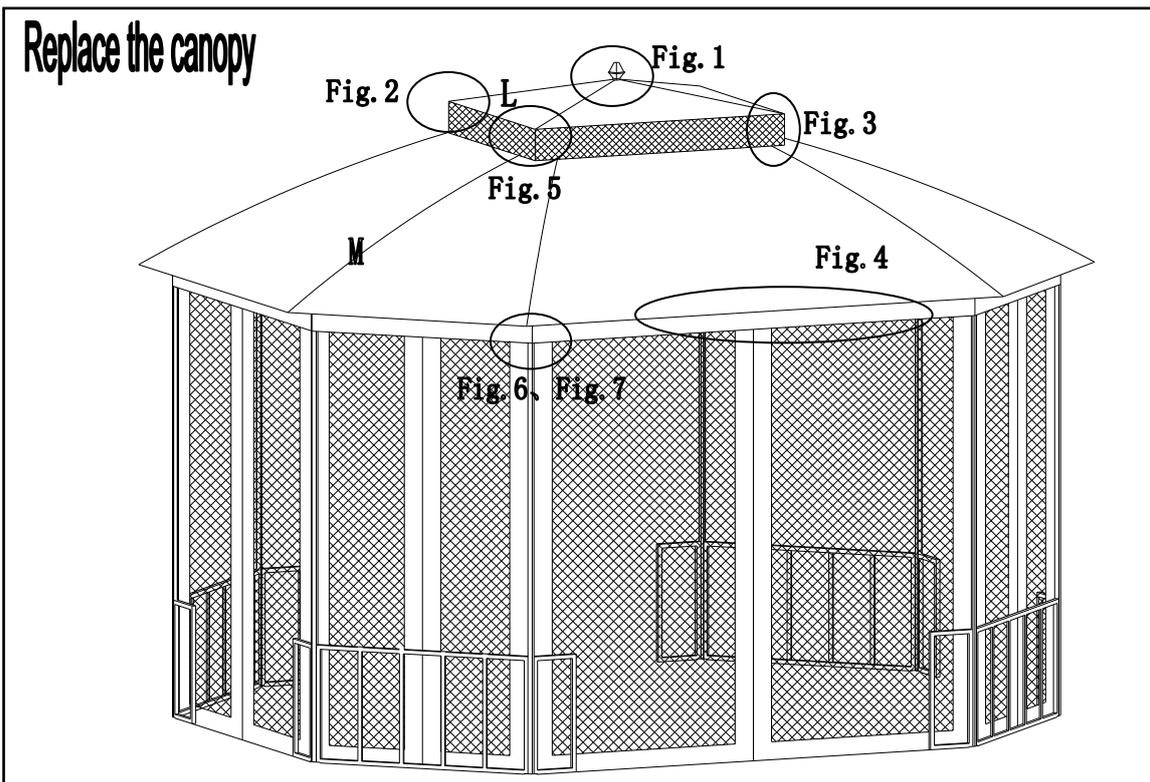
Fig.1: Put the small canopy (L) onto the small top, and then fix the finial (B1) to small top.
