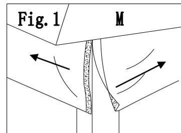
Fig.2: Remove the Big canopy (M) from the big top cant beam (E1).
