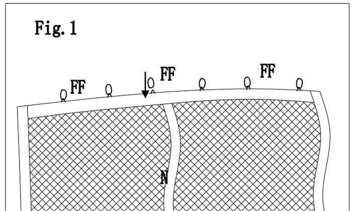
Fig.2: Hang the mosquito netting (N) to the hanging pole by plastic ring (FF).
