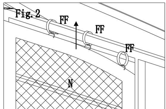
Fig.3: Fix the elastic string and buckle of the netting (N). Tie the tieback to draw the netting in.
