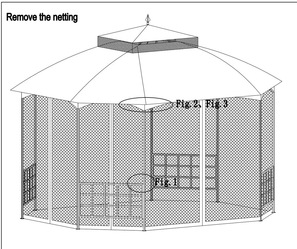
Fig.1: Loosen the elastic string of the netting (N) and the tieback which is fixed on the post.
