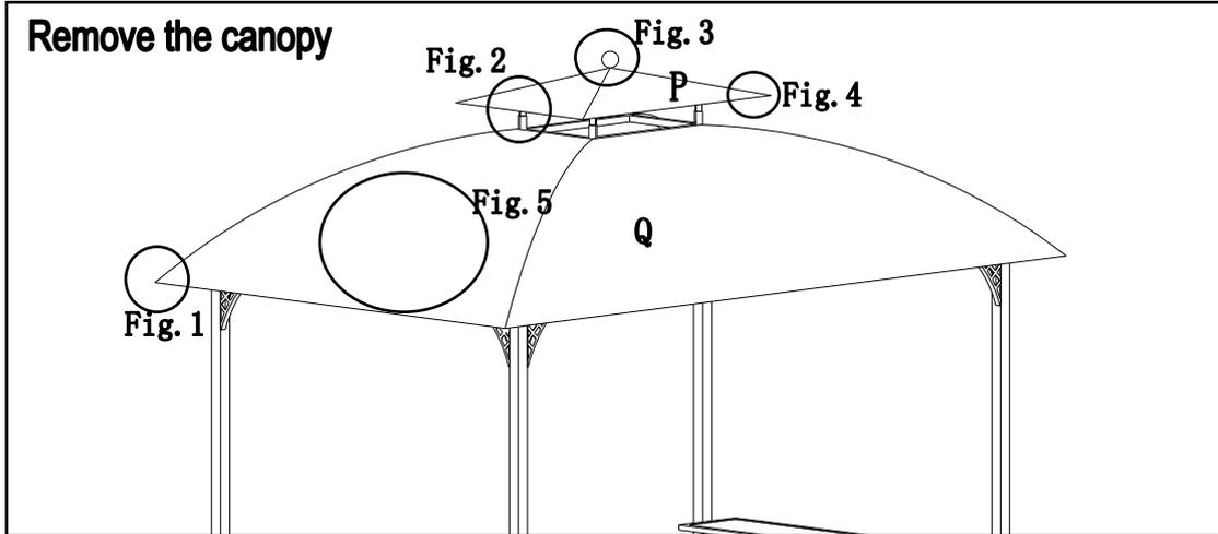
Fig.1: Remove the canopy (Q) from four corners and put the canopy away.
