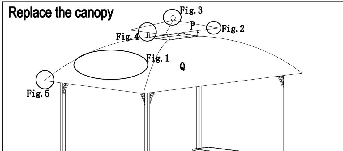
Fig.1: Put the big canopy (Q) onto the big top and do not spread out.
