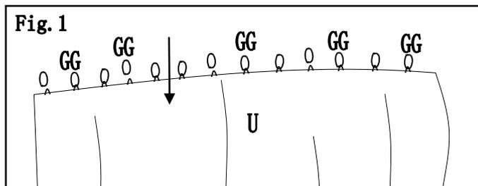
Fig.2: Hang the curtain (U) to the outer side of netting pipe (N, O). (Remark: Long side of curtain should contain 7 plastic ring and short side 6 plastic rings.)
