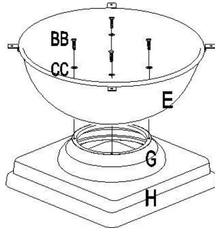
**Step 5:** Put Slate top (D) upside down on a soft, non-abrasive surface, connect assembled base to slate top (D), tighten with bolt (BB) and washer (CC).
