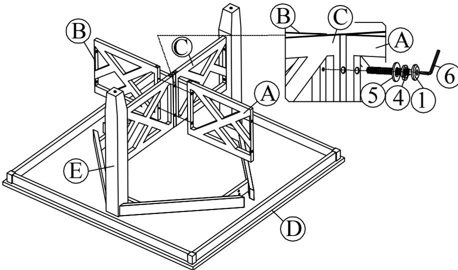
Step 2: Attach Metal Plate A (A) and Metal Plate B (B) to the Metal Plate C (C) by inserting Long Bolt (1), Lock Washer (4), Flat Washer (5) as picture shown. Tighten all Bolts with Allen Key (6). Do not fully tighten.
