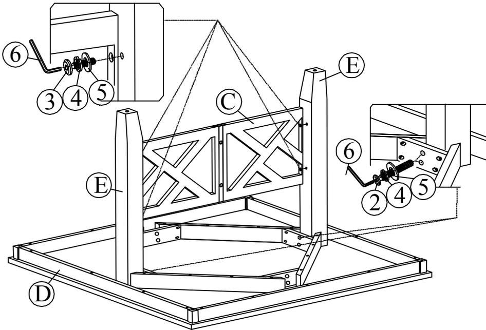
Step 1: Place the Table Top (D) upside down on floor with a piece of cloth or carpet underneath to prevent finish from scratching.
