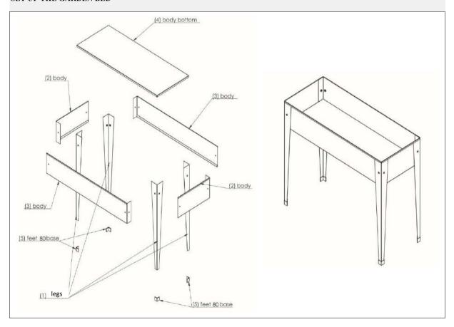
Secure all the parts by 8 Screw Unit (6). Tighten all the screws.
